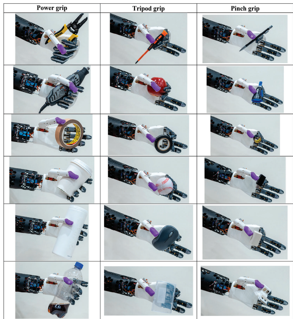
Figure 24. Persistence arm gripping different objects of various shapes, weights, and sizes.
