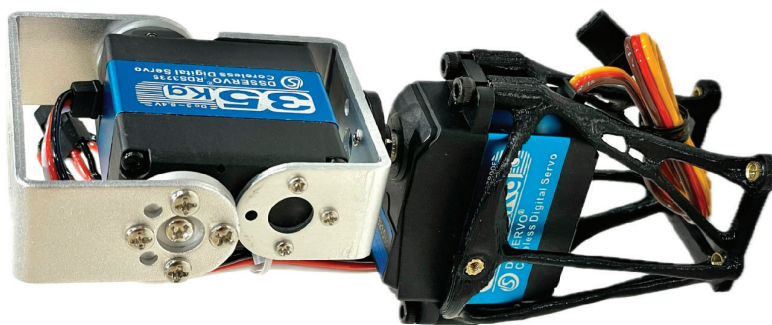
Figure 14. Manufactured wrist actuation mechanism.
